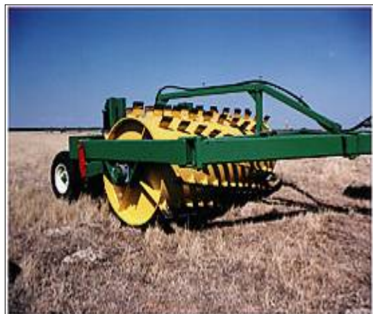
Figure 5.16 Soil aerator implement
