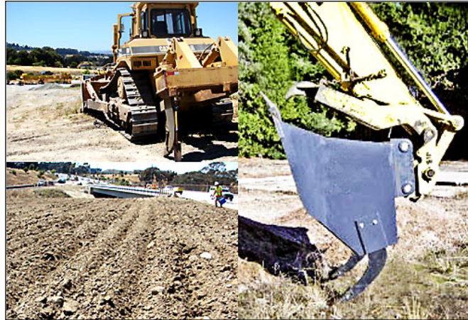
Figure 5.15 Soil aerator implement
