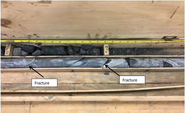
Photograph 3: B-4: Core Run 2 (See Photo No. 1).
