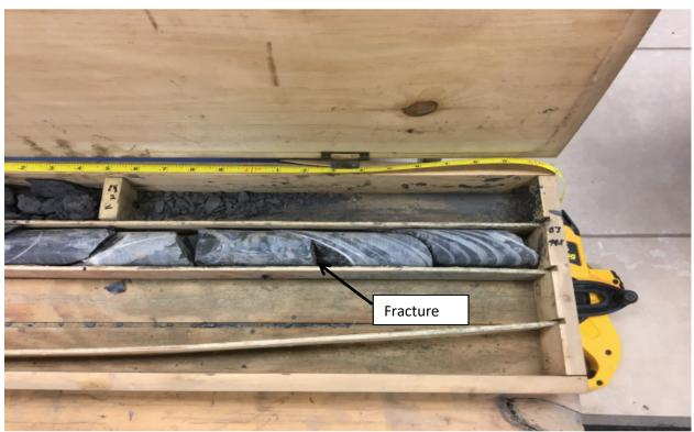
Photograph 4: B-3 Bottom of Core Run 1 – 97.5' – 98.5' (See Photo No. 1). High angle fracture at 97.8'
